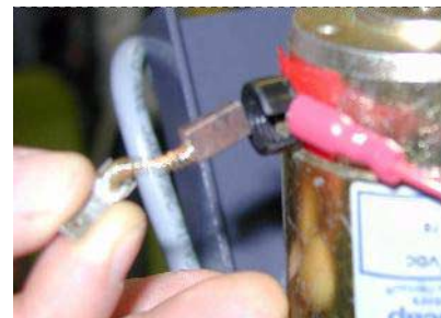
Unscrew the nut and pull on the terminal to remove the carbon.
