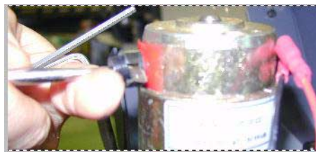
Unscrew the nut and pull on the terminal to remove the carbon.
